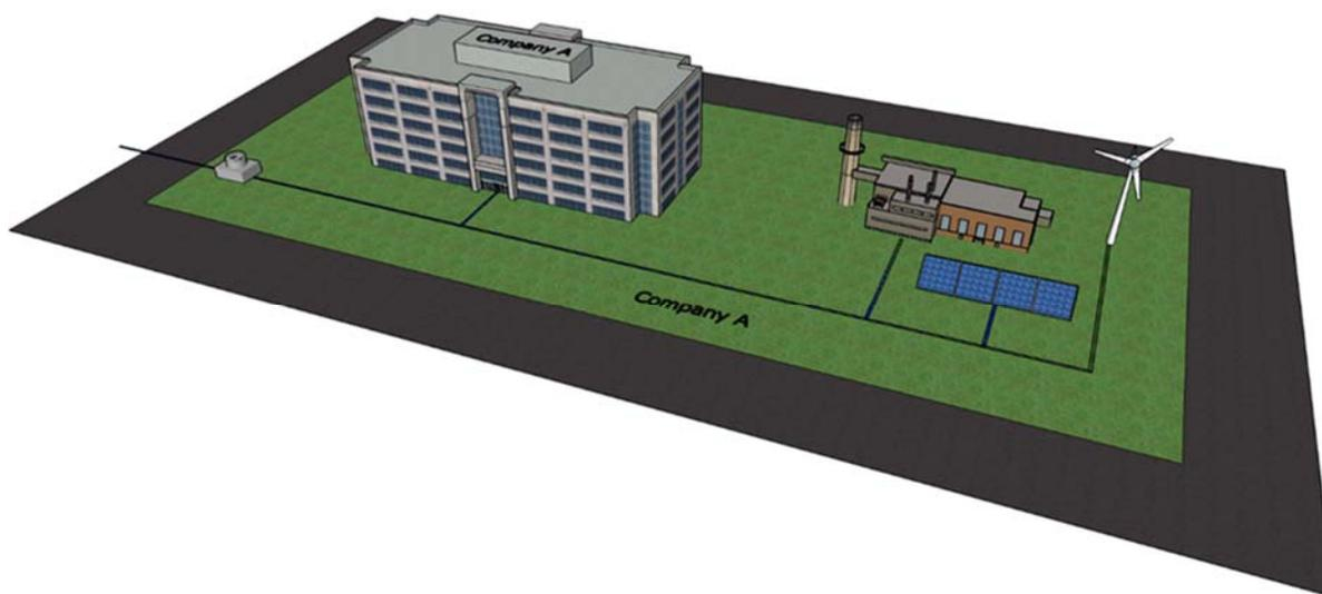
In this scenario, a single legal entity owns and operates distributed generation assets and distributes electricity from such assets on a single continuous property. The microgrid is connected to the macrogrid at a single point of connection.
