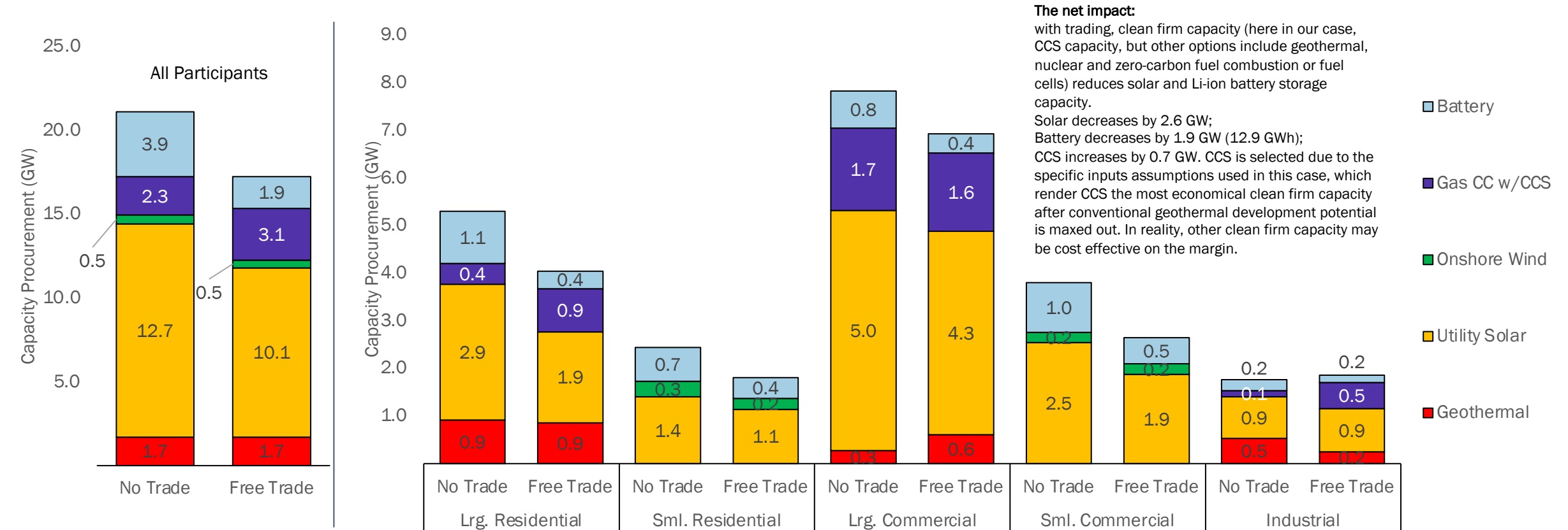
Figure K-4: Capacity procurement of the five modeled California 24/7 participants with or without T-EAC trading. CFE Score Target = 98% for all participants.
