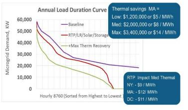
Overall, the operational energy cost savings generated from deploying this technology suite and islanding capability ranges from 40 to 60%. See the adjacent figure for a summary of all of the value or savings categories.
