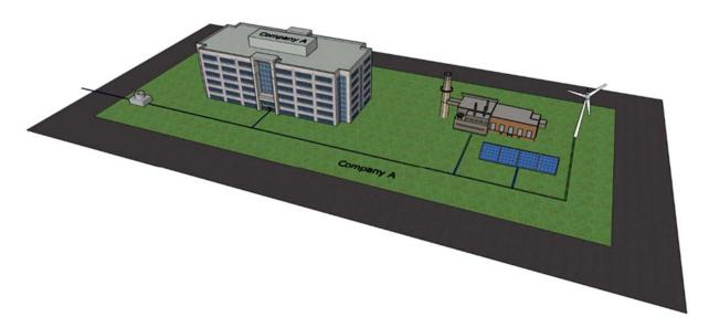
In this scenario, a single legal entity owns and operates distributed generation assets and distributes electricity from such assets on a single continuous property. The microgrid is connected to the macrogrid at a single point of connection.
