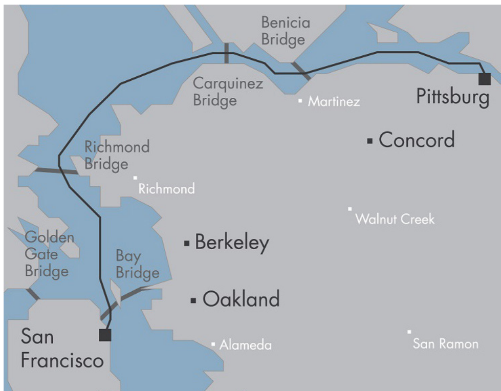
The Trans Bay Cable runs for 53 miles under San Francisco Bay, providing transmission between two PG&E substations. | SteelRiver Infrastructure Partners
